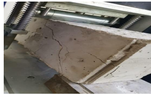
Figure 12. Beam B4 (U-section) Cracks
