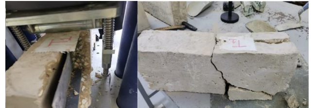
Figure 13. Beam B2 (inverted T-section) Cracks.
