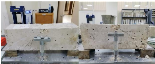
Figure 10. Control beam Cracks
