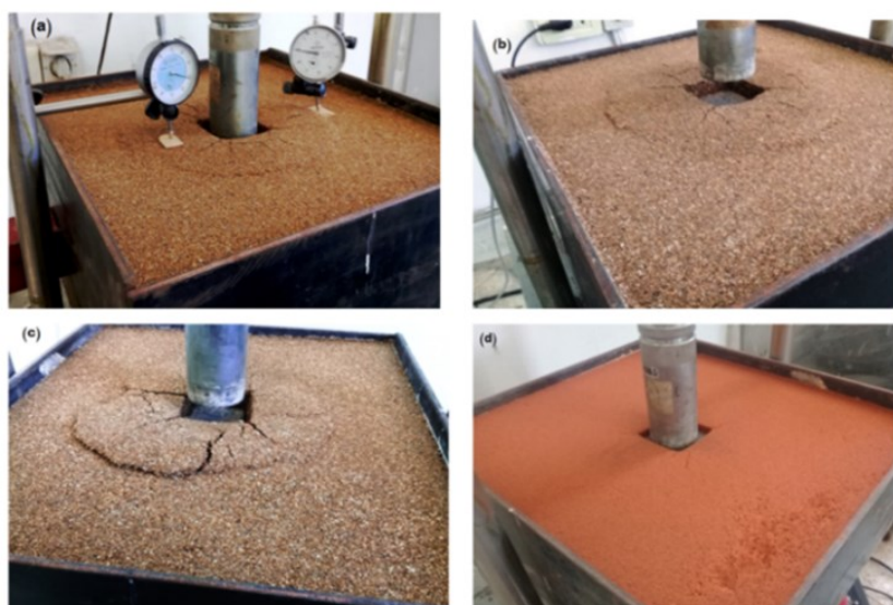
Figure 11. Images of The Bearing Capacity Test at Which General Shear Failure Occurred.
