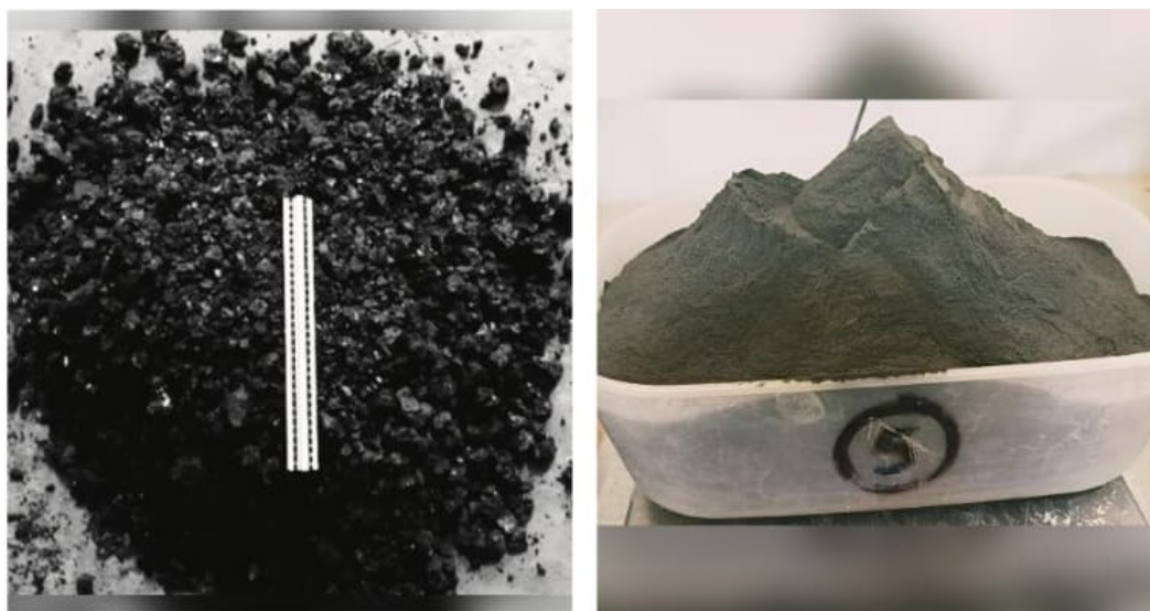
Figure 2. Slag Before and After Grinding
