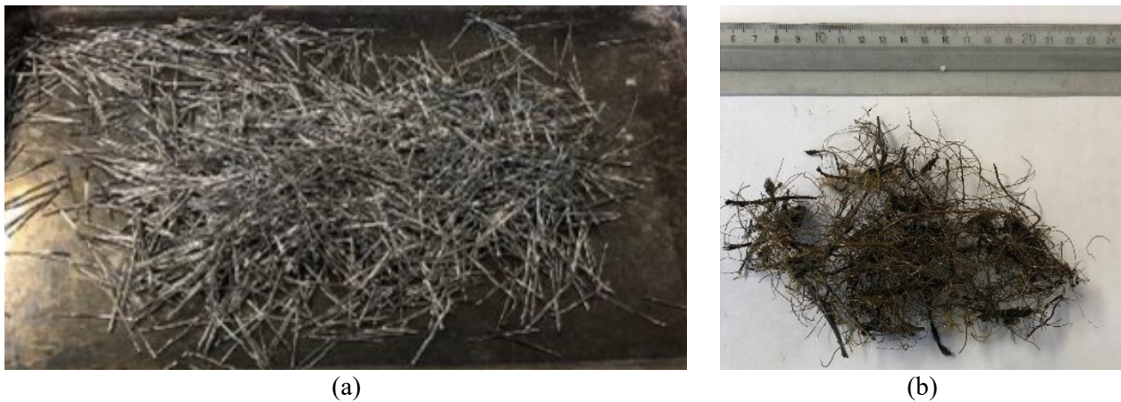
Figure 2. Steel Fibers: Commercial (a) and Recycled (b).
