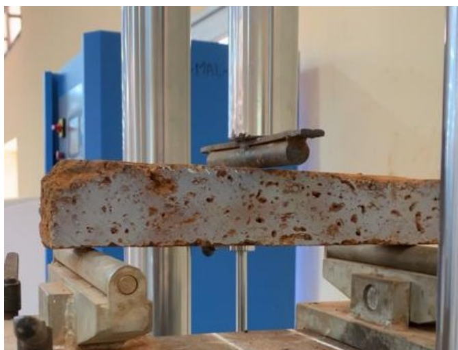
Figure 6. 3 Points Bending Test LS were Dried at 60\pm 2 °C Until Reaching Constant Mass.
