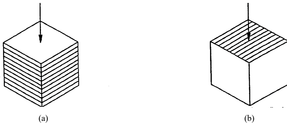
Figure 7. Loading Pan Depending on the Anisotropy Plan. (a) Parallel to Anisotropy Plan. (b) Perpendicular to Anisotropy Plan.
