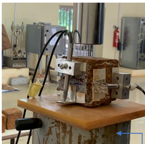
Figure 5. Unconfined Compression Test
