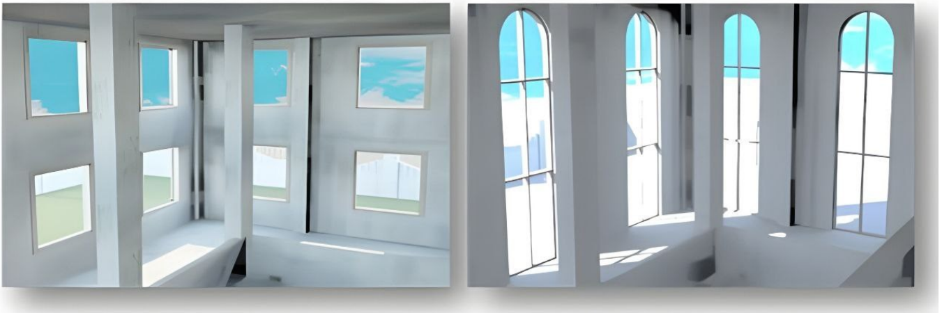
Figure 13. Comparison of Interior Daylight Distribution Between the Two Design Alternatives.
