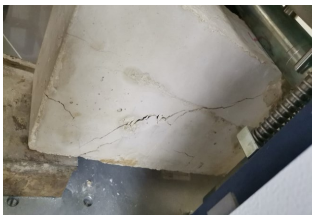
Figure 11. Beam B3 (I-Section) Cracks
