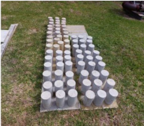
Figure 6. Array of Concrete Cylinders in Outside Exposure Condition
