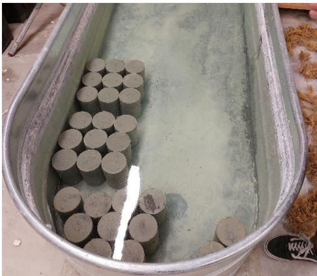
Figure 4. Samples subjected to 28 Days of Curing in a Curing Tank
