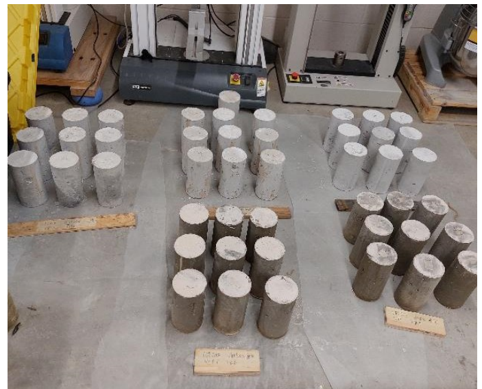
Figure 5. Array of Concrete Samples Placed in Lab-controlled Conditions.
