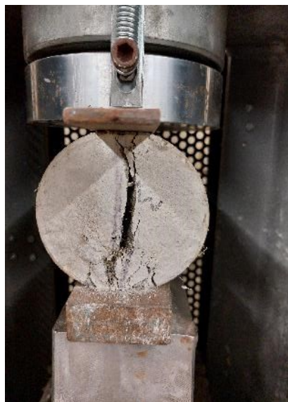
Figure 8. Split Sample from the Splitting Tensile Strength Test
