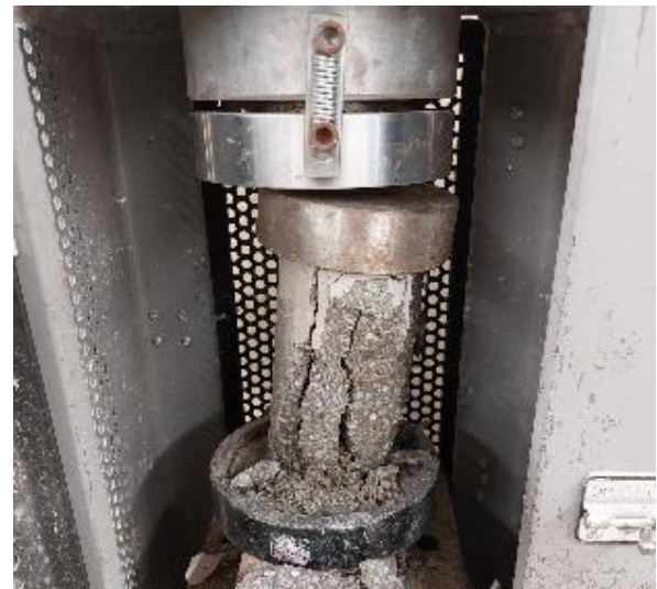
Figure 7. Crushed Sample from Compressive Strength Test
