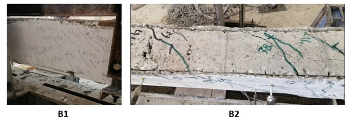
Figure 8. The Difference of the Cracks' Width Between B1 and B2 Beams.
