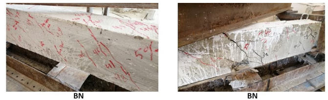
Figure 7. The Cracks Propagation in BN Beams
