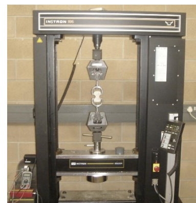
Figure 4. Tensile Test Setup
