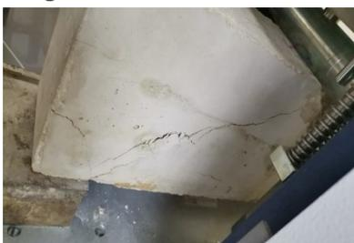
Figure 11. Beam B3 (I-section) Cracks
