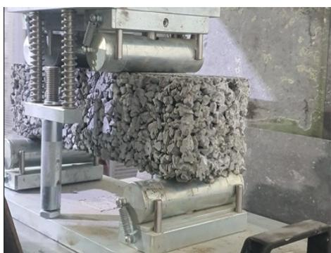
**Figure 6.** Flexural device
