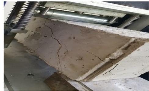
Figure 12. Beam B4 (U-section) Cracks
