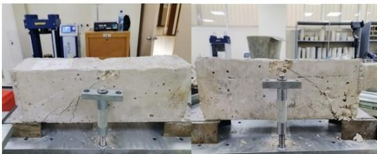
Figure 10. Control beam Cracks
