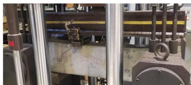
**Figure 1.** Beam Dimensions, Reinforcement Details, and Test Setup Under Two-Point Loading (Ghali et al., 2023).
