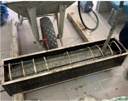
Figure 1. Vibration of concrete inside the molds.
