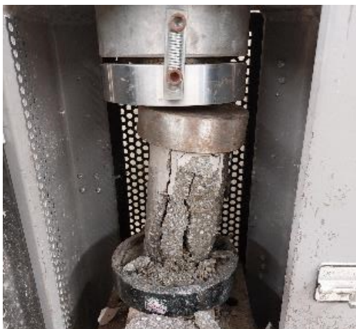
Figure 4. Crushed Sample from Compressive Strength Test
