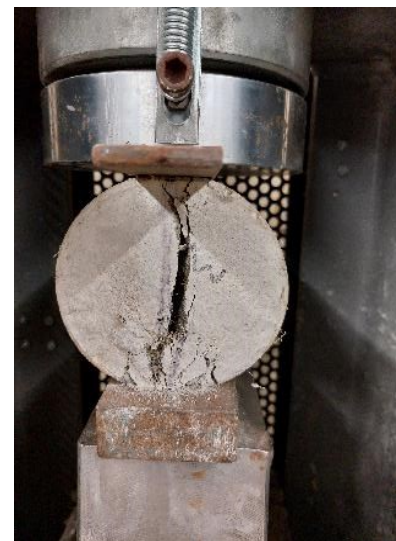
Figure 5. Split Sample from the Splitting Tensile Strength Test
